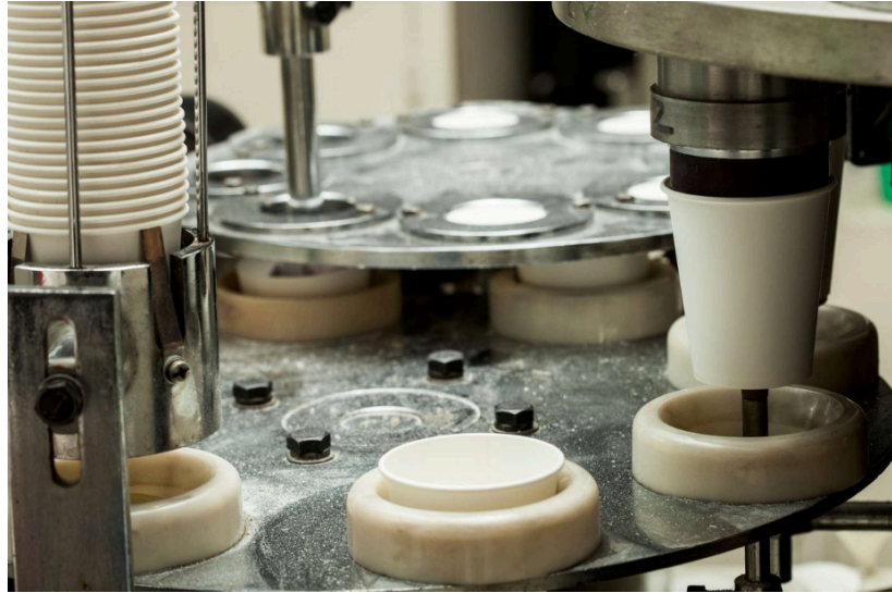
Figure 4 - Shaping Paper Cups (GreenFeel, 2023)
